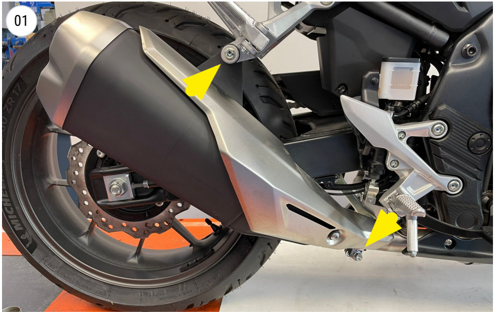
unscrew and remove the stock muffler
