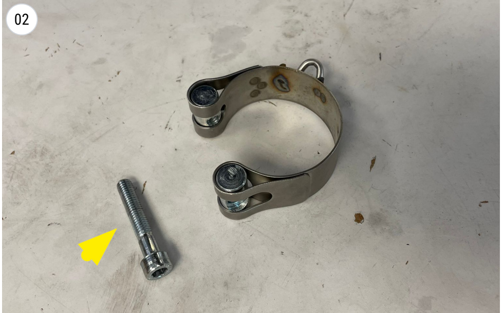
remove the screw to simplify assembly
