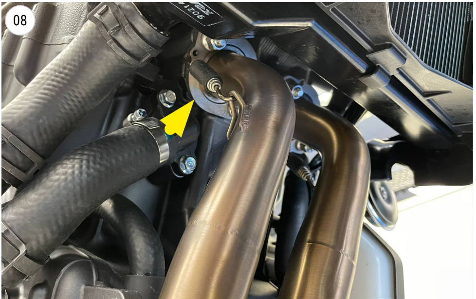
Fit the primary pipes
