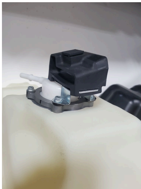
Fig. 3 ( IMS recommends running the larger zip-ty through the slotted holes on the black cover, and then underneath the seat hook style bracket to ensure the cover does not detach )
