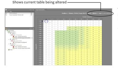
Most maps from Dynojet will include a base Target AFR table. These settings are intended to deliver optimal performance while still maintaining decent fuel mileage in the cruise area (for most models).
