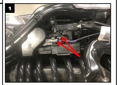
3. Plug the Low Rider Integrated Taillight Harness into the rear turn signal lighting connectors shown in Picture 1. The Low Rider Integrated Taillight Harness JAE turn signal connectors with the brown wire will connect to the Black JAE connectors of the bike's wiring harness. The Low Rider Integrated Taillight Harness JAE turn signal connectors with the Purple wire will connect to the Gray JAE connectors of the bike's wiring harness as shown in Picture 2.
