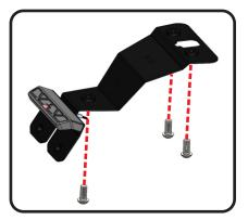
3. Install *FE-LP-BKT*, license plate bracket using the *M6X12FS-SS*, flat head screws.
