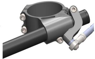
4) Sit on the motorcycle and rotate the handlebars lock to lock. Be sure that you have full handlebar travel in both directions before operation. Check the damper for freedom of motion throughout the entire range of travel.
