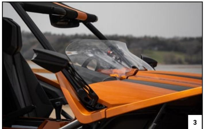
8. Insert the tabs of your new Klock Werks Flare® into the dash and set it into place (FIG 3).
