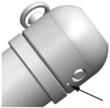
4) **Nut Side:** The small base with the expansion slot will be installed in the right of the axle itself. To install the base, thread the 8x25mm socket head bolt into the assembly until it is almost tight, leaving a small gap between the halves. Slide the assembly into the hole of the axle and be sure that it is fully seated against the axle.
