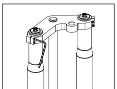
Loosen the clamping screws in the upper clamp.
