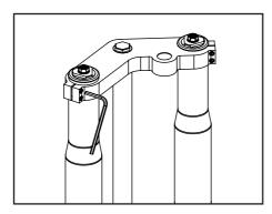
Tighten the upper fork clamp bolt to manufacturer's specification and adjust preload and damping settings to previous or recommended settings. (Located at the front of document)
