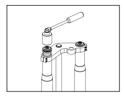
With the bike supported under the bottom fork clamp unscrew both fork caps with either Tool No. 113-010-020 or a top cap socket
