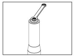
Remove all the preload from both forks using the 14mm hex in the centre of the top cap.
