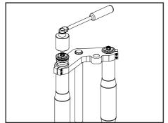
With one person on each handlebar slowly lift the bike and support the bike under the **bottom fork clamp** so the wheel is off the ground. Refit the top caps to the fork legs and torque load to 10N/m (7.35 lb-ft) - using Tool No. 113-020-000
