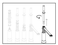
Remove the piston rod pull up tool.
