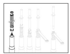
Refit the preload tube with nylon seats, with the holes facing downwards along with the optional spring you are choosing to use and the nylon spring pusher.
