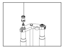
If a large amount of oil has been lost removing the spring it is necessary to check the oil level. To do this you will need to remove the spring preload spacer from under the main spring using a wire hook.
