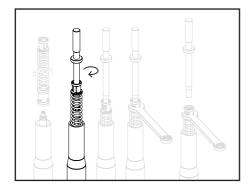
Using the pull up rod - Tool No. 113-030-015 screw this onto the piston rod joiner.
