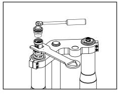
Fit the top cap onto the piston rod joiner using Tool No. 113-010-020 and a 14mm socket. Tighten the top cap to the piston rod joiner torque load to 20N/m (14.75lb - ft).
