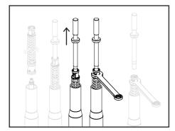
Pull the piston rod up and locate Tool No. 113-010-020 through the nylon spring pusher onto the 17mm hex on the piston rod joiner.
