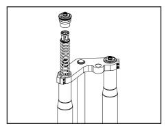
Remove the nylon spring pusher and the main spring slowly, keeping as much oil in the fork leg as possible.
