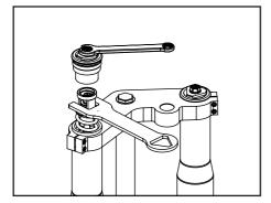
Remove the top cap nut assembly from the piston rod joiner using a 14mm spanner and Tool No. 113-010-020.
