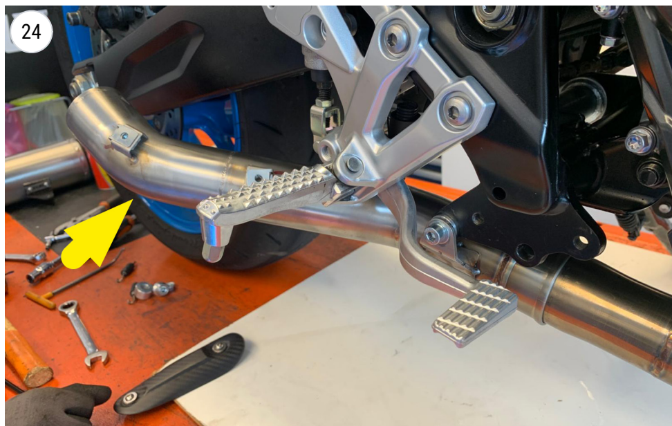
INSTALL THE FINAL PIPE
