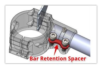
CRITICAL IMPORTANCE: The replacement handlebars (part number 13-4104) for this kit have a groove for the set screw and retention spacer to engage. DO NOT USE THIS CLIPON ASSEMBLY without all of these components. A handlebar without a groove for these two retention components will not work. Failure to heed this warning could result in serious injury or death.
