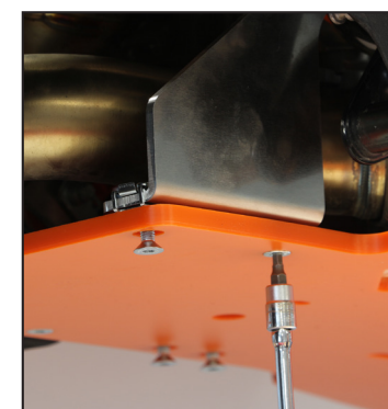
14 Place the 4 TFHC 6x25mm screws (2 on each side of the skid plate) and tighten them all.
