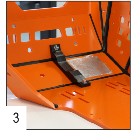
3 Place the HDPE block using 2 TFHC 6x25mm screws + M6 washers and EM6F bolts.
