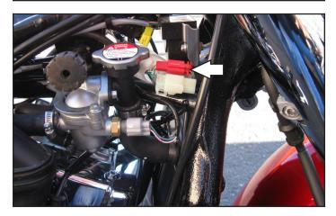
14 Plug the set of RED, 2-pin connectors of the PC6 wiring harness in-line with the bike's Crank Position Sensor connectors.
