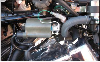
17 Plug the set of GREEN colored wires of the PC6 inline with the BLUE/YELLOW wire and the coil.
