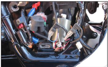
Locate and unplug the Crank Position Sensor connectors on the right hand side of the bike, up by the steering stem.
