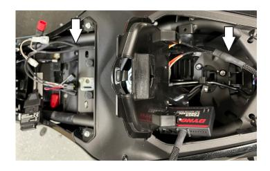
2 Lay the PC6 in the tail section and route the harness down the right side of the bike going towards the throttle bodies.
