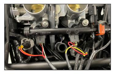
10 Plug the PC6 in-line of the stock wiring harnes and injectors.
