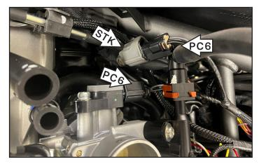
12 Plug the PC6 in-line of the stock wiring harness and TPS.
