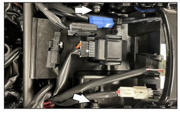
6 Unplug the crank position sensor connector.
