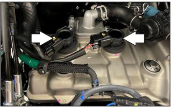
13 Unplug the stock wiring harness from each ignition coil stick.
