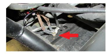
Secure the ground wire with the small ring terminal to the stock common ground bolt on the frame located behind the driver's seat.
