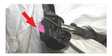
Gently pry at the small, purple tab at the top of the connector. Slide tab outwards to release the wires.
