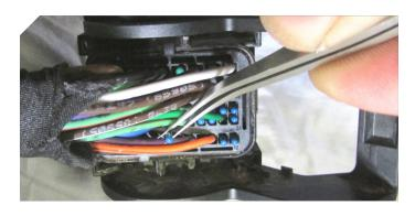
Pull the small blue seal out of it. Gently insert the pinned wire of the APM switch into position #18 until it is latched in place.
