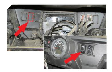
After installing the swtich in the desired location, route the cable to the ECM compartment located behind the driver's seat.
