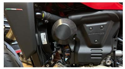
2) Attach the slider bases to the motorcycle using the 12mm bolts provided, threading them in place of your motor mount bolts. The longer base goes on the left side with
