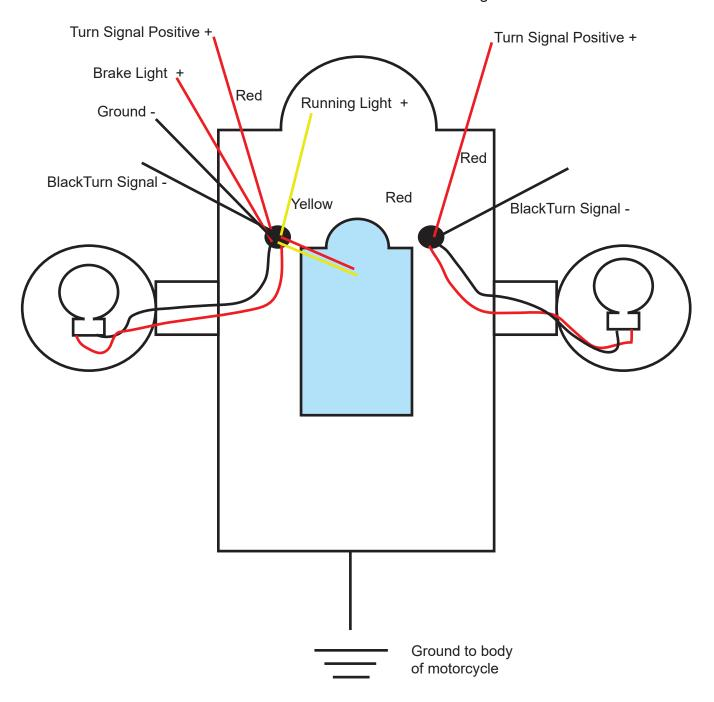
This light will not function if the mounting bolts are not creating a ground to the body of the motorcycle!
