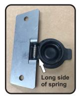
2. Place 13961-FEBKT-1, key cover bracket under 13961-FEBKT, fender bracket. Using a small flathead screwdriver, pull the long side of the spring up and slide the key cover bracket so it catches the edge of the fender bracket as shown.
