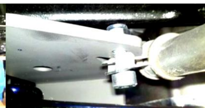
Figure 1.8 Use 6mm bolt and lock nut to hold brake clamp to bracket
