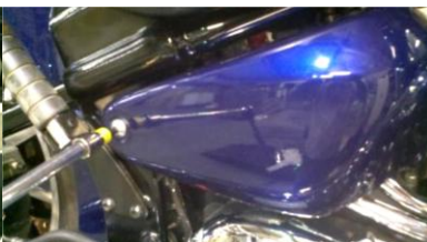
Figure 1.4 Remove right side panel using a 5mm hex key wrench
