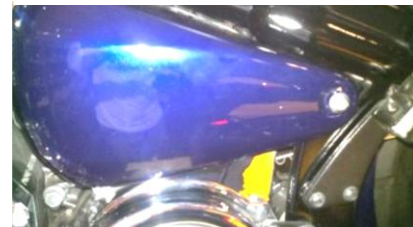
Figure 1.2 Remove cover using a 5mm hex key wrench
