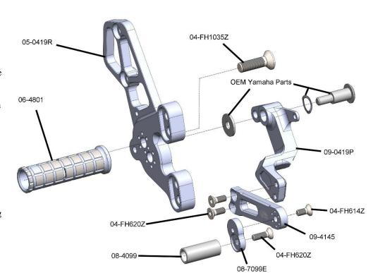
6) Bolt the brake bracket assembly to the frame using the OEM hardware.
