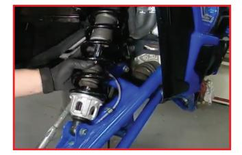
Set "zero Preload" by pressing down on a-arm and holding to fully extend internal bump stop spring. Rotate preload ring clockwise until spring stack contacts preload ring.
