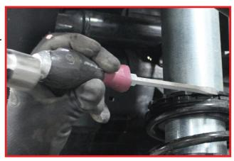
Rotate OEM preload rings counter clockwise all the way to top of threaded shock body. OEM spring stack is now loose.
