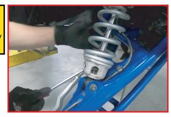
Loosen OEM upper preload ring from OEM lower preload ring. Use flathead screwdriver and hammer or mallet.
