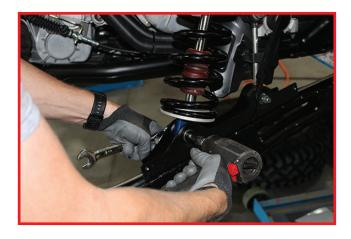
Set "zero Preload" by pressing down on trailing arm and holding to fully extend internal bump stop spring. Rotate preload ring clockwise until spring stack contacts preload ring.
