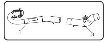
7. Install (No. 5) *left muffler*, over (No. 3) 22843-144/744, left tailpipe outlet. Align muffler mount bracket to muffler mount and secure using the stock muffler mount bolt and washer. Torque to factory specification.
