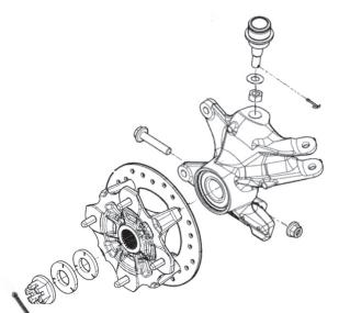
Remove the cotter pin, axle nut, and washers from the hub assembly, then remove the hub. (30mm)
