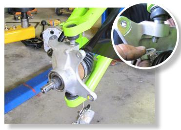
Secure the upper arm at the knuckle using the factory washer and nut. Install the cotter pin.
