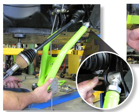
Connect the hub at the LOWER pinch bolt FIRST, then slide the axle through AFTER. (19mm)
