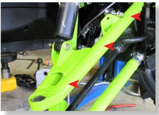
Route the brake lines down the FRONT of the upper control arm. Secure them with the 133B brake line clamps
