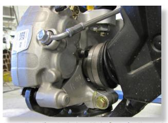
Secure the caliper to the knuckle by fastening the stock caliper mounting bolts. ENSURE THERE IS NO PINCHING OR BINDING OF THE BRAKE LINES.
