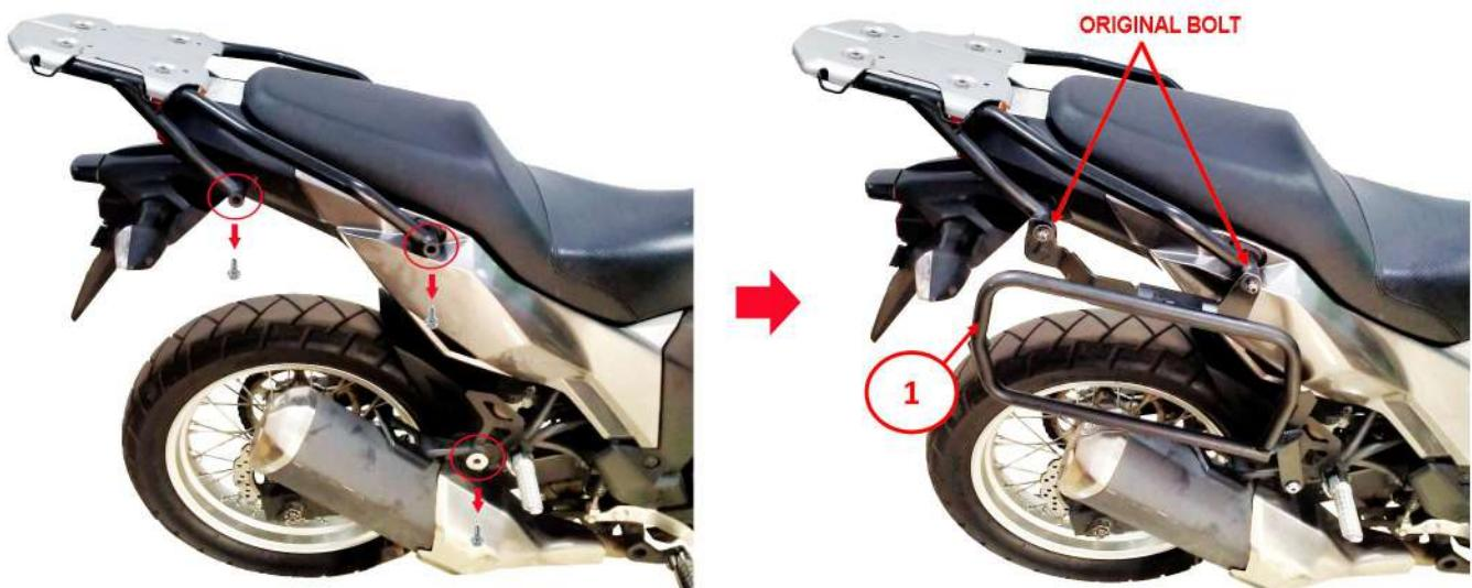
Remove the original bolts from motorbike and install 4P bracket with original bolt and parts no. 2, 3, 4
