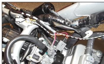
9 Unplug the stock connector from the TPS located on the left side of the throttle body.
