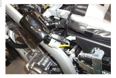
3 Unplug the stock Crank Position Sensor connectors.
