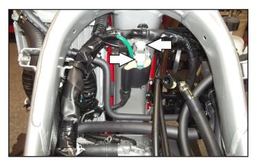
12 Unplug both of the stock wires from the Ignition Coil.
