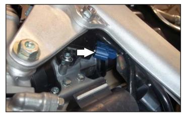
8 Unplug the crank position sensor connector.
