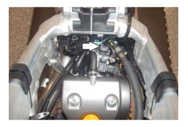
4 Unplug the stock wiring harness from the injector.
