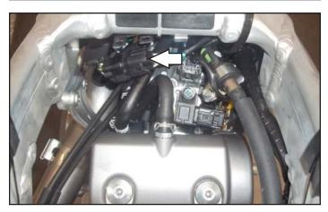
9 Plug the PC6 in-line of the stock wiring harness and crank position sensor connector.
