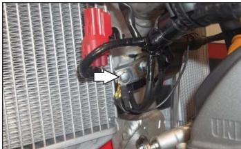
10 Plug the PC6 wiring harness in-line of the ignition coil and the stock coil wires.
