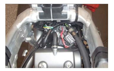
5 Connect the PC6 in-line of the stock wiring harness and the injector.
