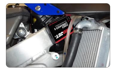
5 Install the PC6 module to the right hand side of the frame using the supplied Velcro and/or the zip tie.
