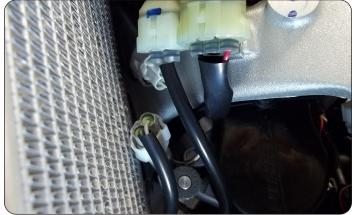
17 Remove the 2 bolts that secure the left radiator to the frame.
