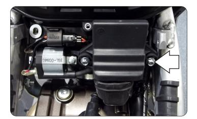
4 Remove the right ECU bolt, and pull the ECU loose from its mounting location.
