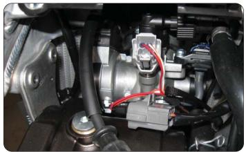
10 Remove the 2 radiator mounting bolts on the right hand side of the bike.
