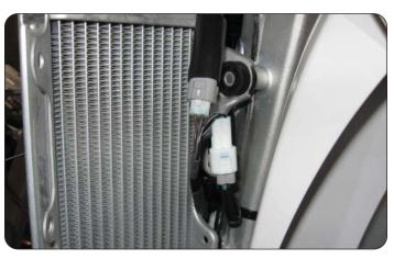
12 Plug the PC6 harness in-line of the stock wiring harness for the Throttle Position Sensor connectors.
