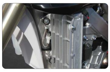
14 Plug the PC6 harness in-line of the stock wiring harness for the crank position sensor connectors.
