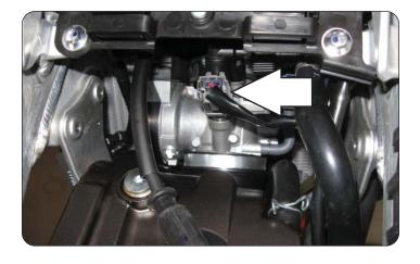
5 Unplug the stock wiring harness from the fuel injector.
