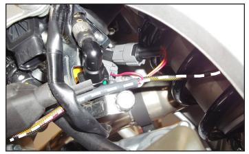
6 Locate and unplug the Secondary Fuel Injector.
