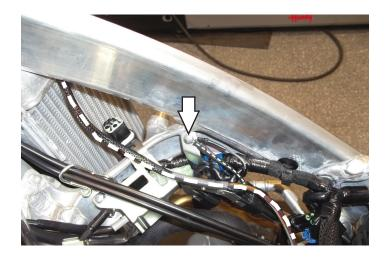
3 Secure the PC6 ground wire with the small ring terminal to the frame using the stock common ground bolt.
