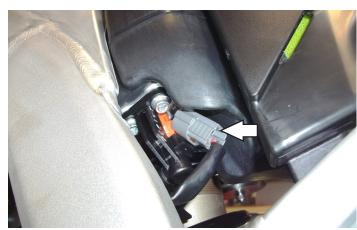
7 Plug the pair of PC6 wiring harness leads with YELLOW colored wires in-line of the secondary injector and stock wiring harness.
