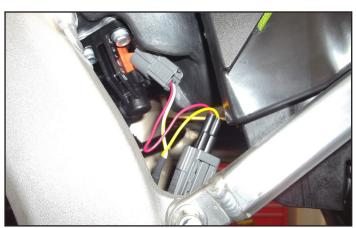
8 Pull back on the rubber boot covering the Throttle Position Sensor connector to expose the stock TPS wires.
