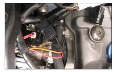
8 Plug the PC6 wiring harness in-line of the stock TPS connectors.
