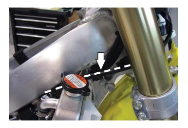
4 Continue to route the PC6 harness down the right side of the bike. Route the harness to the inside of the frame and go towards the throttle body.
