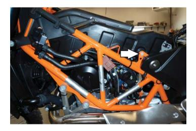
Remove both of the screws (one on each side) that secure the air box to the frame.
