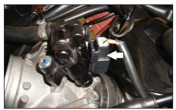
9 Plug the PC6 wiring harness in-line of the Fuel Injector and the stock wiring harness.
