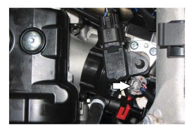
4 Unplug the stock wiring harness from the Fuel Injector.
