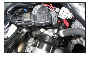
5 Plug the **PC6** in-line of the bike's Fuel Injector and the stock wiring harness.
