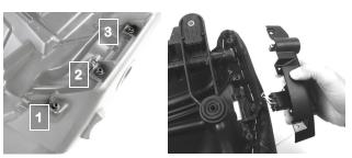
Unplug electrical connector attached to heat switch (if equipped), behind switch plate.
