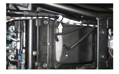
6 Route the PC6 harness along the stock main harness up to the throttle body.
