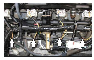
9 Attach the connectors from the PC6 wiring harness to the stock wiring harness and injectors as shown.
