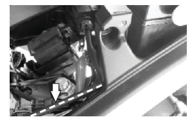
7 Route the PC6 harness along the left hand side of the battery and inside the fuel tank frame bracket, as shown, or under the fuel tank if it was not removed.
