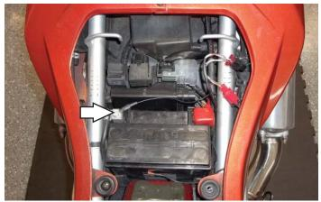
8 Locate and unplug the stock sub-harness connector for the bike's Fuel Injectors.
