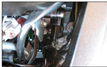
11 Install the PC6 module in the tail section.
