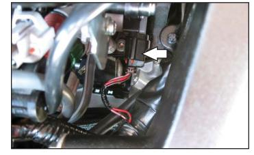
10 Plug the 3 pin connectors from the PC6 in-line of the stock TPS and wiring harness.
