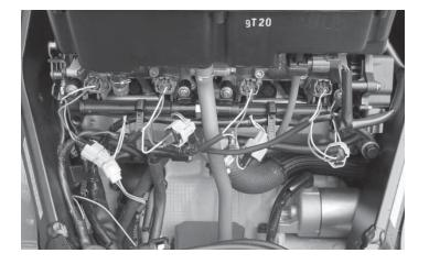
7 Plug the connectors from the PC6 in-line of the stock fuel injectors and the stock wiring harness.
