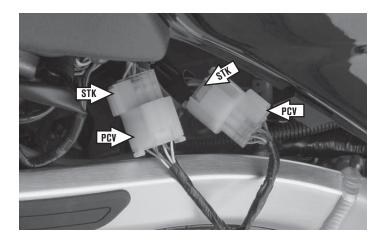
4 Plug the pair of connectors from the PC6 in-line of the stock connectors.
