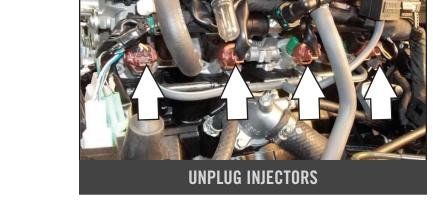
9 Plug the PC6 wiring harness in-line of each fuel injector and the stock wiring harness.
