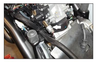
On the left side of the rear throttle body, locate and unplug the lower primary Throttle Position Sensor.
