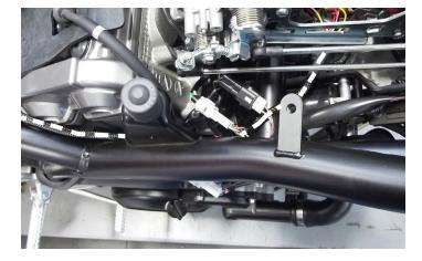
7 Plug the pair of PC6 connectors with BROWN colored wires in-line of the stock Crank Position Sensor connectors. 8 Locate and unplug both of the stock connector pairs for both of the bike's Ignition Coils.
