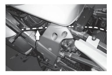
5 Route the PC6 harness under the fuel tank bracket and to the left side of the rear cylinder.
