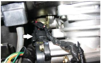
9 Plug the connectors from the PC6 in-line of the stock wiring harness and the TPS.
