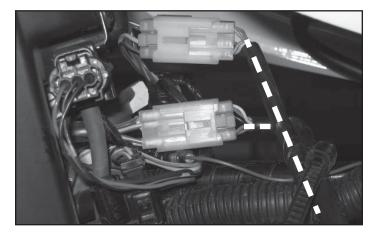
8 Locate and unplug the Throttle Position Sensor. This TPS connector has RED, GREY, and BLACK/BROWN wires and is located on the left hand side of the throttle body.
