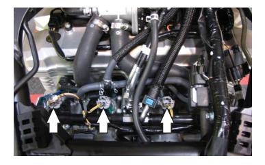
Unplug the stock wiring harness from each of the fuel injectors.
