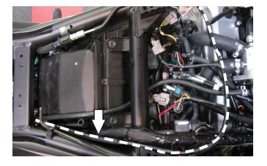
6 Plug the connectors from the PC6 in-line of the fuel injectors and the stock wiring harness.
