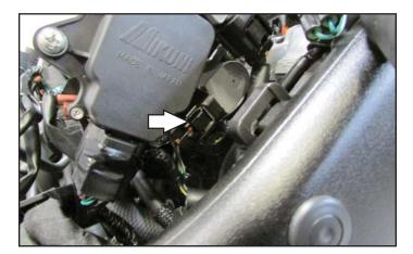
8 Connect the PC6 in-line of the stock TPS and wiring harness.
