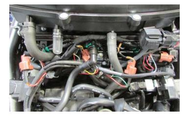
6 Plug the PC6 in-line of the stock injectors and wiring harness.
