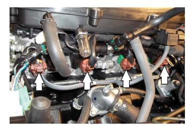
5 Unplug the stock wiring harness from each injector.
