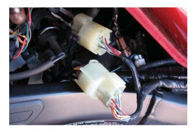
4 Attach the connectors from the PC6 to the stock wiring harness connectors as shown.
