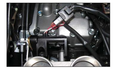
8 Plug the YELLOW colored wires of the PC6 in-line of the stock wiring harness and rear injector.
