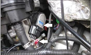
12 Attach the GREY wire of the PC6 to the stock WHITE/BROWN wire of the Throttle Position Sensor using the supplied Positap.
