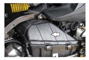
2 Remove the air box cover by releasing the clips around the edge of the air box.
