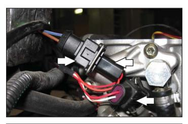
11 Plug the pair of PC6 leads with ORANGE colored wires in-line of the stock wiring harness and the rear fuel injector.
