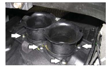
3 To remove the air box base, remove the six bolts around the velocity stacks.
