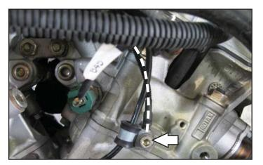
Attach the ground wire of the PC6 to the rear cylinder head on the left side.
