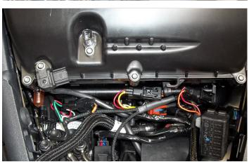
8 Unplug the Crank Position Sensor connector.
