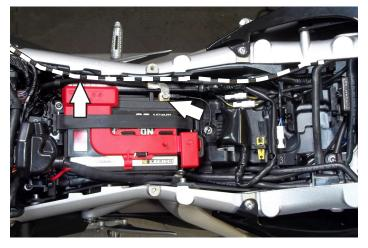
Attach the ground wire of the PC6 to the negative (-) side of the battery.
