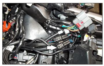
9 Plug the PC6 wiring harness in-line of the Crank Position Sensor and the stock wiring harness.
