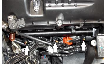
7 Plug the PC6 in-line of the stock wiring harness and each injector.
