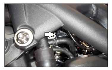
10 Unplug the Throttle Position Sensor connector.
