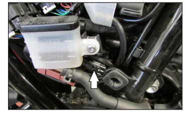
8 Plug the WHITE 2 pin connectors from the PC6 in-line of the stock CPS.
