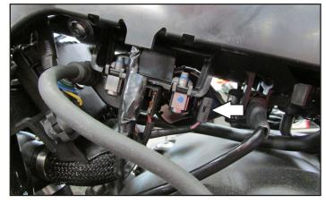
13 Unplug the signal wire of stock wiring harness from the #2 ignition coil.
