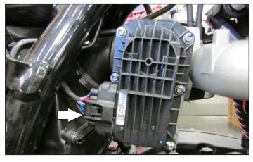
10 Plug the PC6 wiring harness in-line of the stock wiring harness and the Throttle Body Servo.
