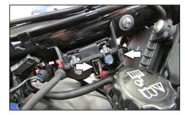
16 Plug the PC6 in-line of the stock wiring harness and ignition coil.
