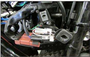
9 Locate the Throttle Body Servo on the right hand side of the motorcycle and unplug the stock wiring harness from it.
