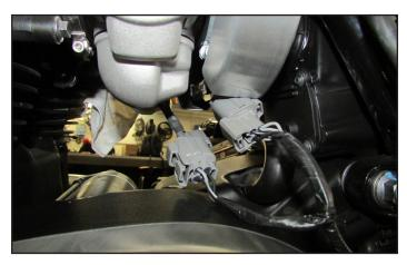
10 Unplug the stock wiring harness from each injector.
