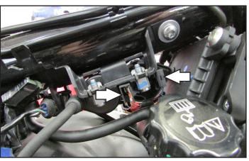
14 Unplug the stock wiring harness from the #1 ignition coil.
