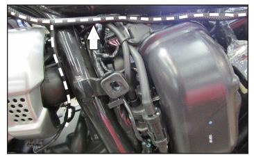
8 Unplug the stock Throttle Position Sensor connector.
